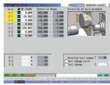
HMI (Human Machine Interface) – Graphics displayed for each item and screens display all the necessary information in one place for operating convenience.
